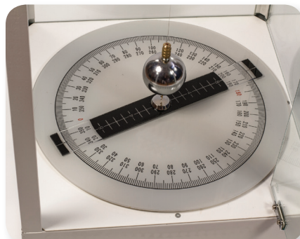
The graduated circle carries an adjustable double-ended marker bar for precise measurement of the plane of swing.
