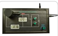
The main unit includes a voltmeter, nanoammeter, and light/voltage adjustment knobs.
