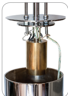
The sample heating assembly can be raised out of the oven on the telescoping support rod.
