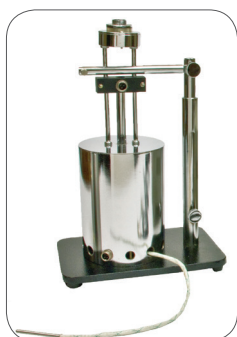
The sample oven contains a cooling fan, a massive metal block with an electric heater, three samples, and a control system sensor.
