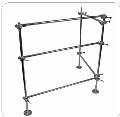
Sections can be added at any angle. This can provide limited stability without securing all of the foot plates to the bench. Add heavy apparatus inside the angle of the sections for stability.
