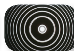
Triple fringes are strong \pi -polarized components that are used for measurement.
